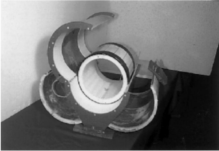
FIG. 8. The prototype four-arc gradient set shown with the RF resonator closed (it is fully openable).
